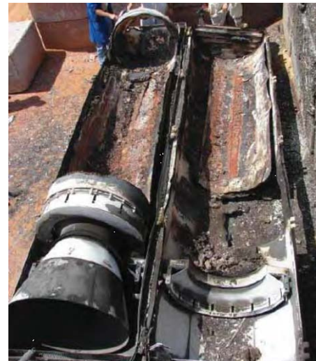
Figure 14. Spartan motor after burn.
