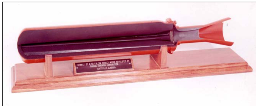
Figure 5. Cutaway model of the M58 Falcon rocket motor.
