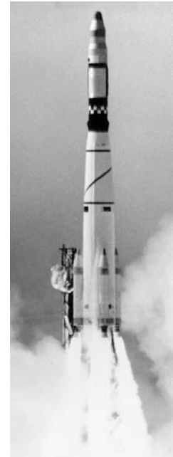
Figure 7. First TAT-AD Launch with three Castor I strap-ons in 1963.
